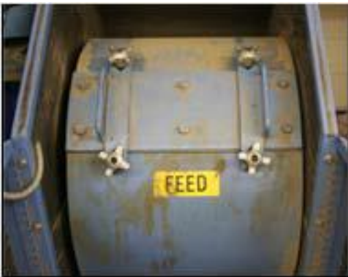
LA Abrasion drum for 300 revolutions without steel spheres
